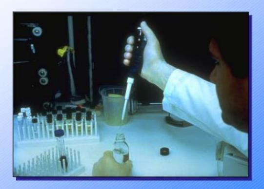
Use mechanical pipetting devices
